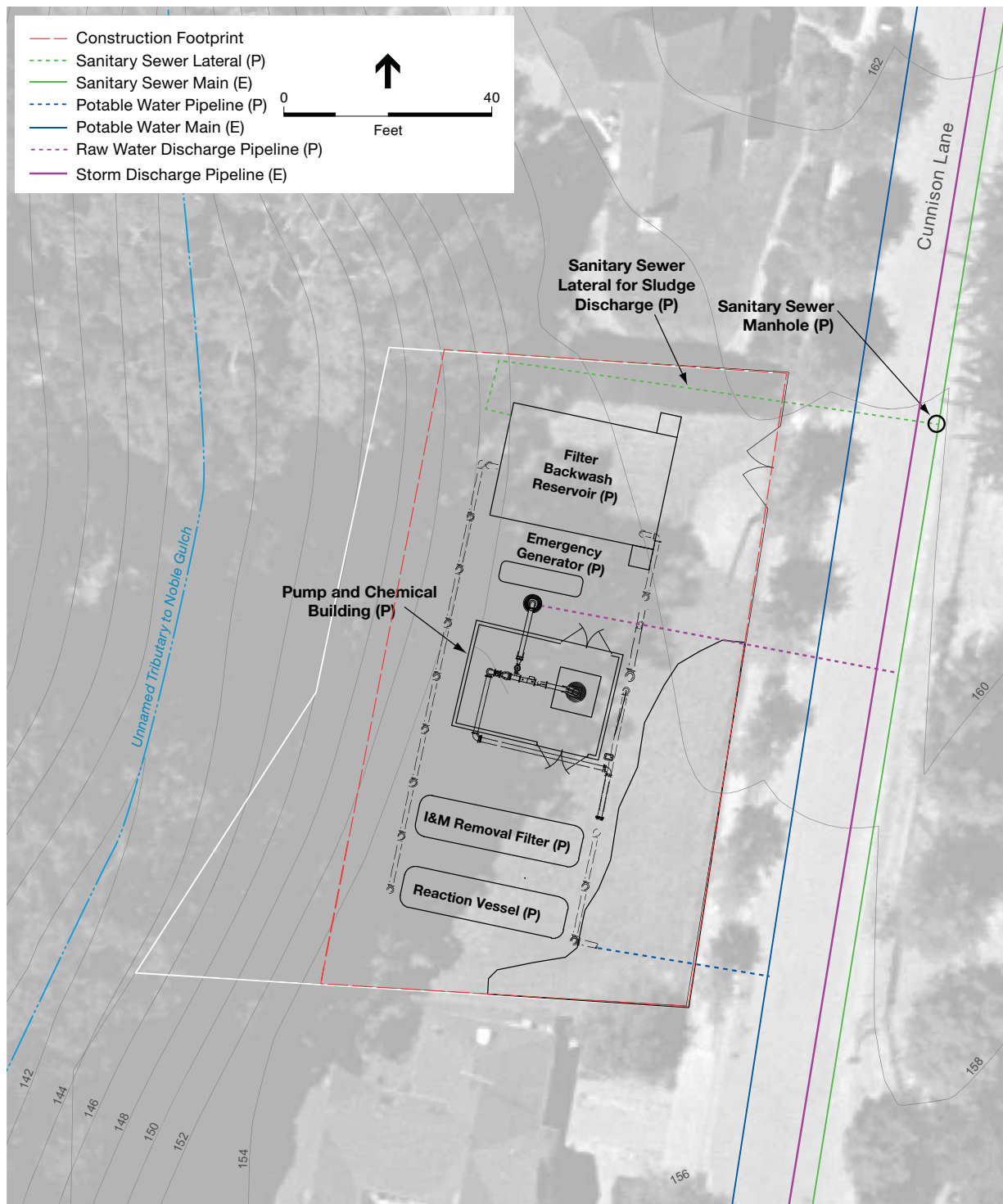
Figure 2-4 Cunnison Lane Well Site Preliminary Site Plan
