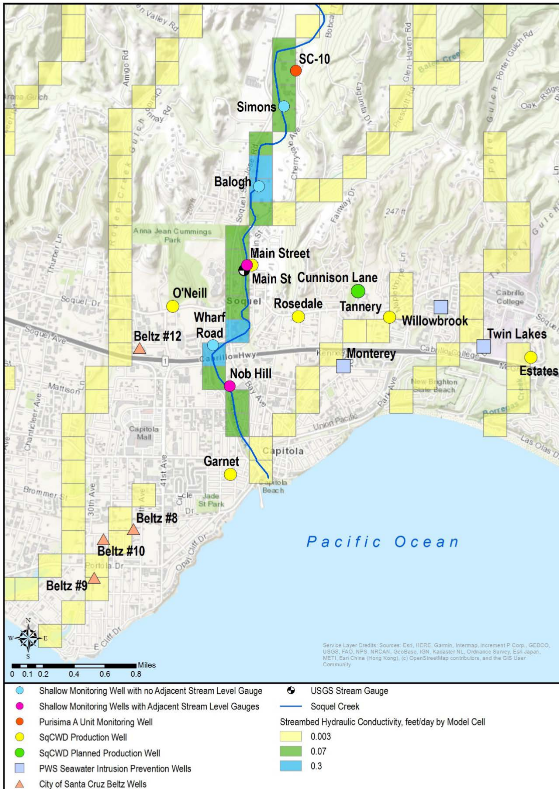
Figure 17. Locations of Monitoring Wells used as Representative Monitoring Points with Groundwater Elevation Proxies for Streamflow Depletion
